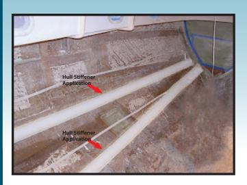
Taco Marine introduces a versatile Hull Stiffener product, which provides a cost effective means of adding additional stiffness to aluminum or fiberglass panels. Easy installation on most wood or fiberglass materials. Construction provides adhesive installation on composite or metal materials. Material can be drilled for fastener use as well.
